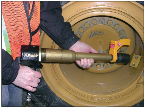
RAD 10GX (12818), 12" nose extension (14195), with reaction arm (13512)
