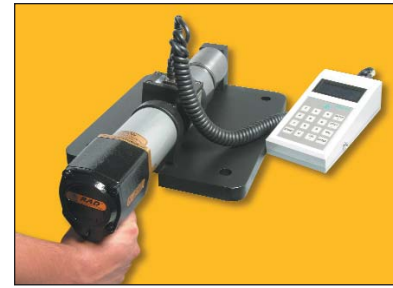
All RAD® pneumatic torque wrenches are individually calibrated on our exclusive "RAD-CAL" dynamic joint simulator torque analyzer
